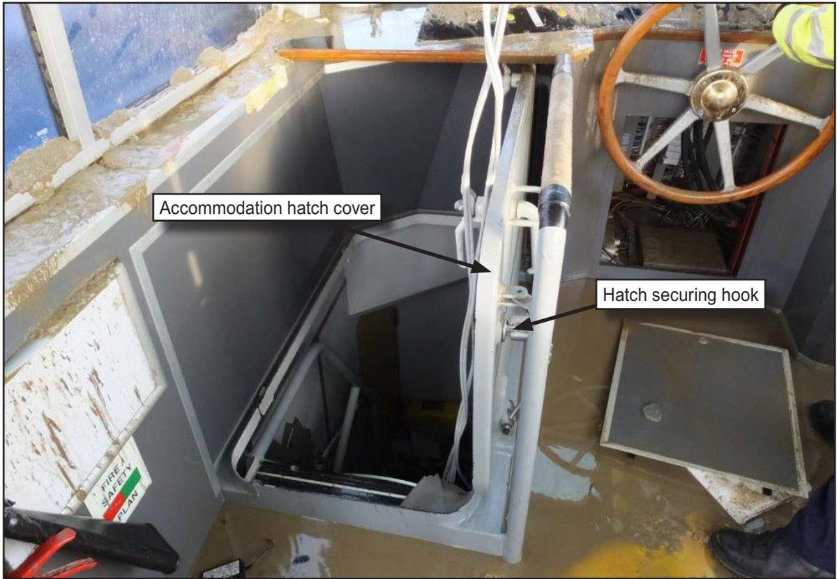
**Figure 4:** Accommodation hatch cover (hooked open)
