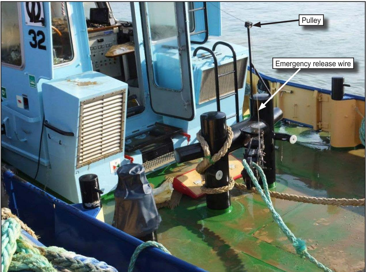
**Figure 9:** Towing hook emergency release wire
