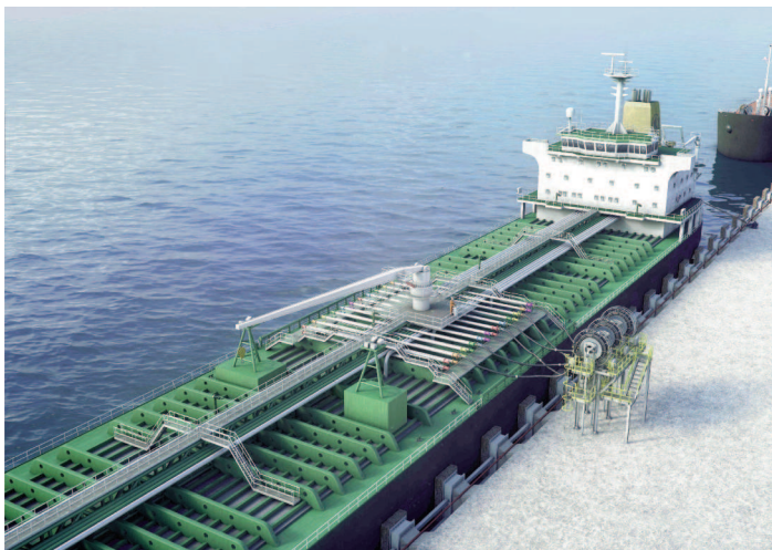
The Quay Reel load/discharge system is claimed to be able to reduce cargo operations time by up to 60%.
