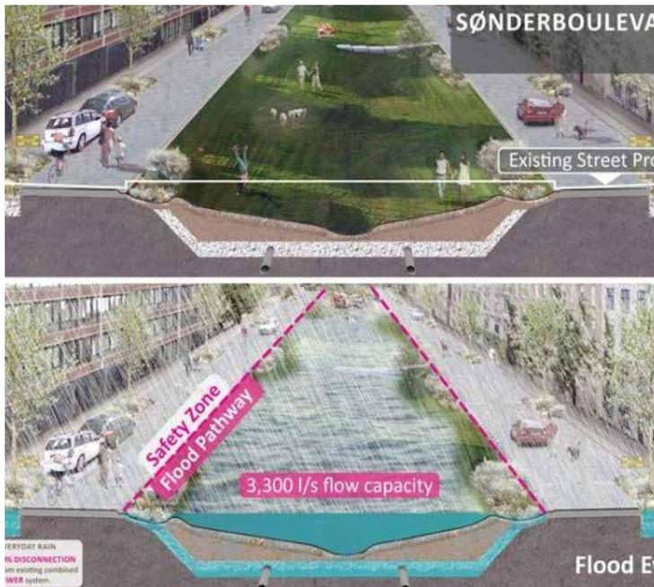
*Green infrastructure can be created in multi-functional spaces that can be used for recreation in dry weather, but provide flood storage in extreme weather. Source: Ramboll*
